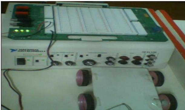
Figure7: Interfacing robot with NI-elvis
